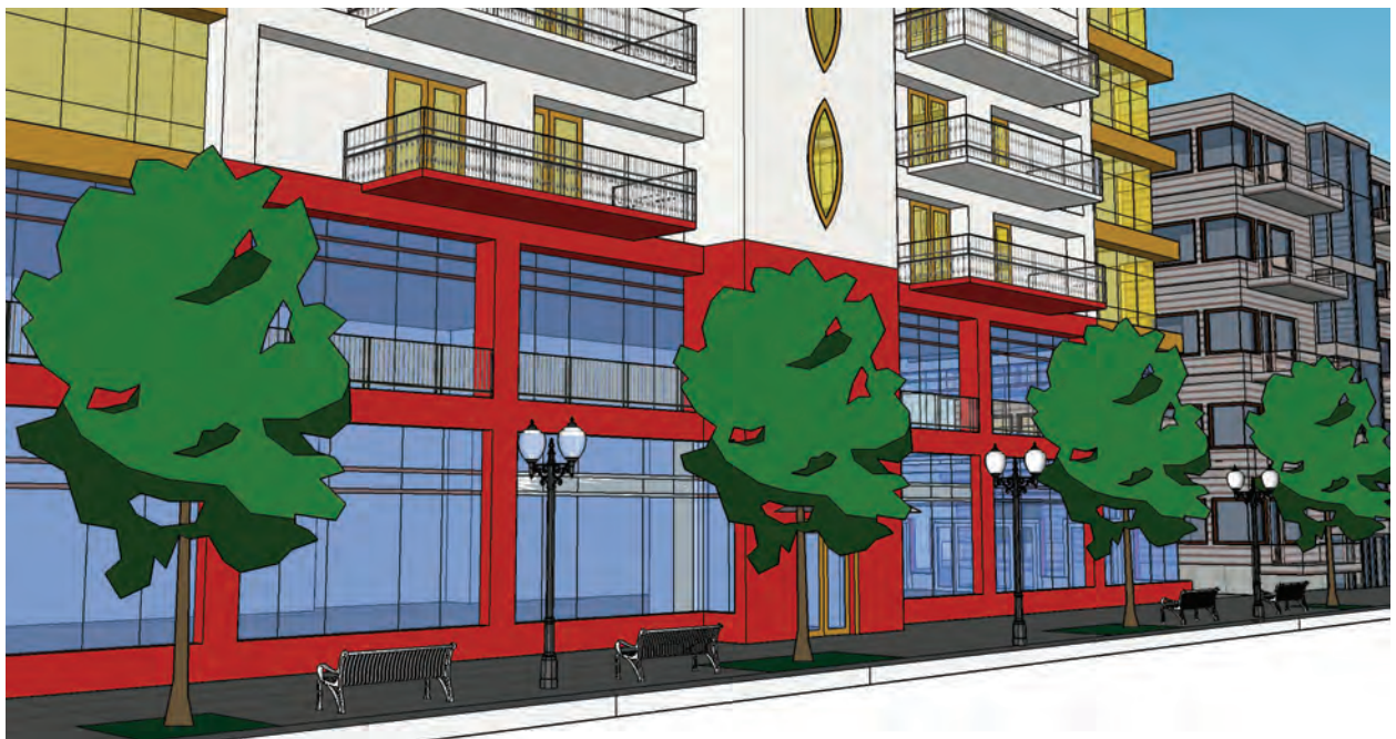
Top: Tree box with an integrated urban bioswale. Bottom: Tree interval 40 feet center to center. Street lights 40 feet center to center.
